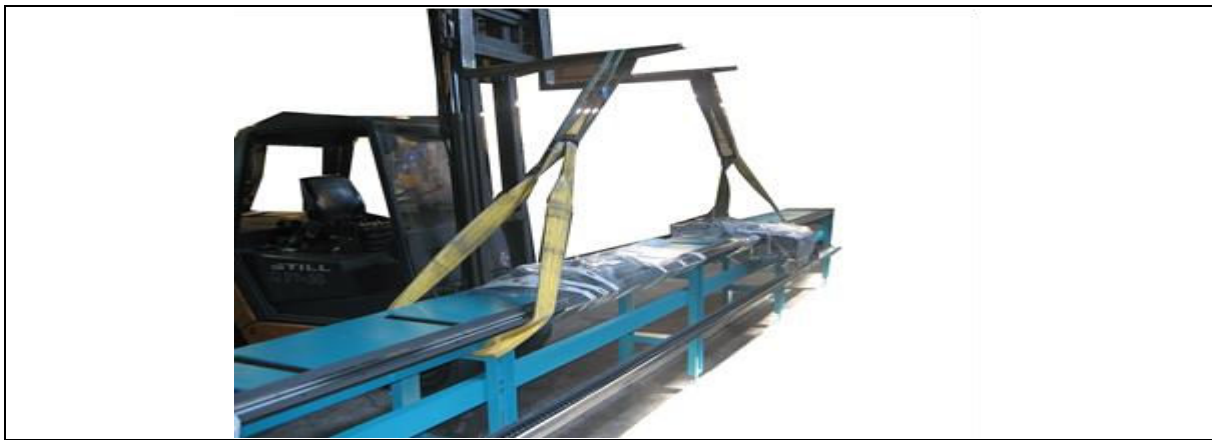
Lifting of a complete system, incl. roller conveyor
